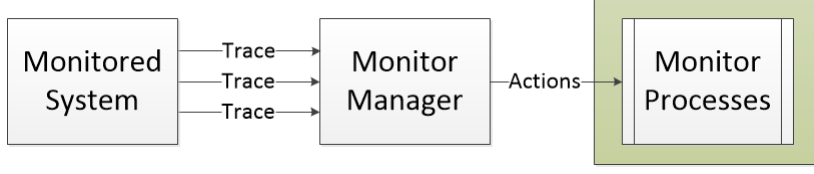
Figure 7: A high level architecture of the monitor
