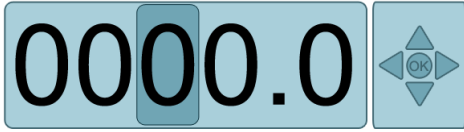
Figure 5: Five button interface frequently used in medical infusion pumps
