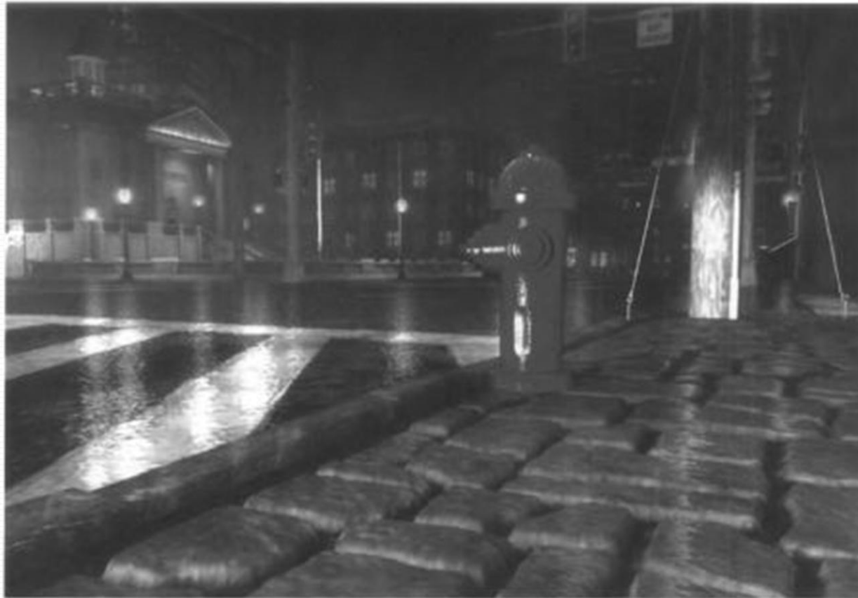
Figure 6.1. Texturing. Color, bump, and parallax occlusion texture mapping methods are used to add complexity and realism to a scene. ( Image from "Toyshop" demo courtesy of Natalya Tatarchuk, ATI Research, Inc. )
