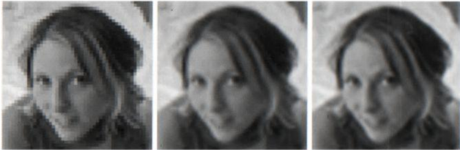
Figure 6.8. Texture magnification of a 48 \times 48 image onto 320 \times 320 pixels. Left: nearest neighbor filtering, where the nearest texel is chosen per pixel. Middle: bilinear filtering using a weighted average of the four nearest texels. Right: cubic filtering using a weighted average of the 5 \times 5 nearest texels.
